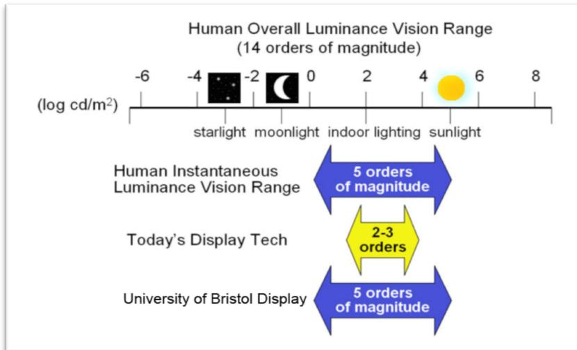
prototype which displays 5 orders. Coincident with this, the BBC in turn have created a 200 frame per second projection system.
