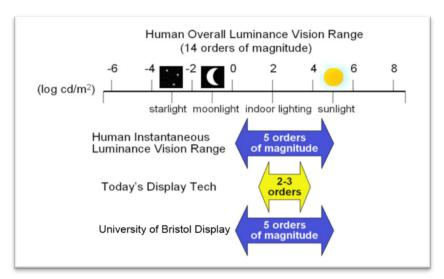
prototype which displays 5 orders. Coincident with this, the BBC in turn have created a 200 frame per second projection system.
