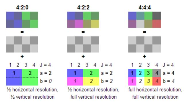
One unheralded change that HDMI 2.0 brings is an ability to send 4:2:0 content natively. Previous HDMI versions only used 4:2:2 or 4:4:4 subsampling, even though the Blu-ray format uses 4:2:0, so content first needed to be converted to 4:2:2 or 4:4:4. With UltraHD pushing the bandwidth limits of HDMI, Version 2.0's ability to send bandwidth-saving native 4:2:0 content, and to do so without degrading image quality, is a benefit.
